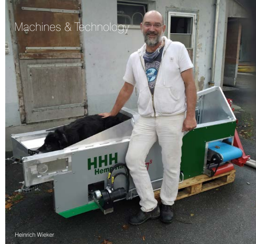
Front-mounted, the HHH 700 can harvest hemp continuously in the field.
