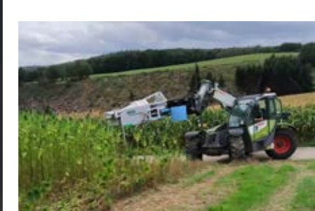
Front-mounted, the HHH 700 can harvest hemp continuously in the field.
